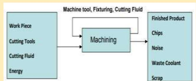
**FIG 2: Input-Output diagram of a machining process**
