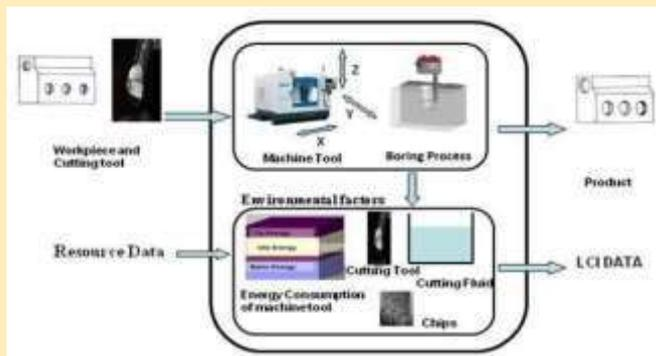
FIG 3: LCI DATA FOR MACHINING PROCESS
